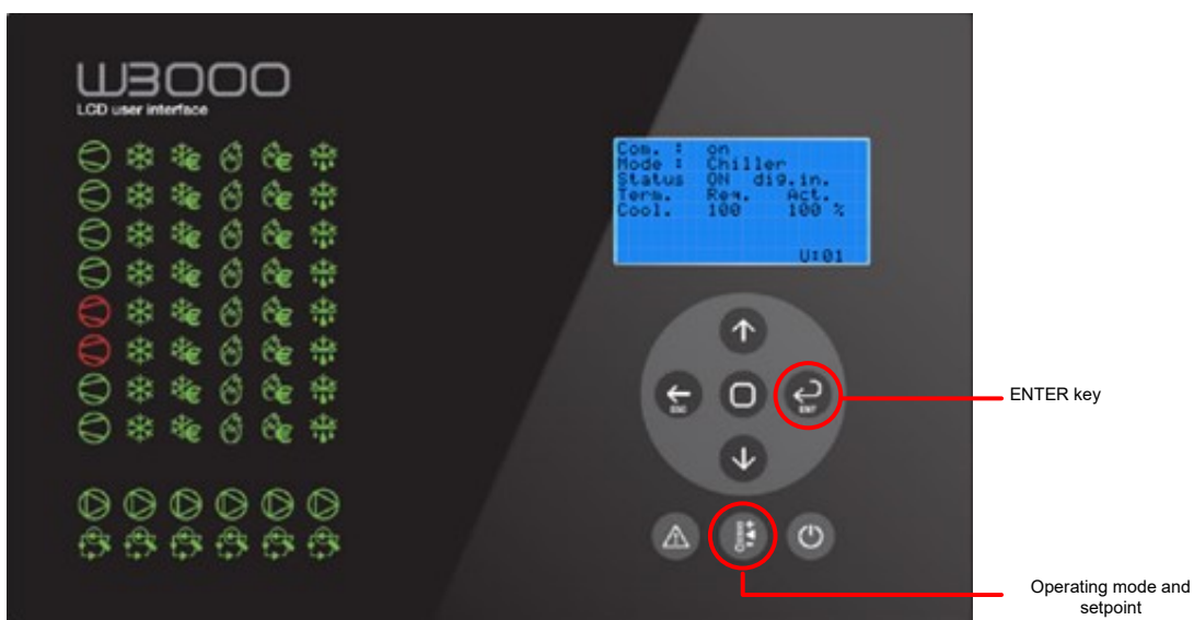
Figure 8.7: buttons for changing operating mode and confirmation (ENTER).
