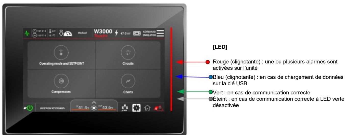
Figure 8.9 : description LED.
