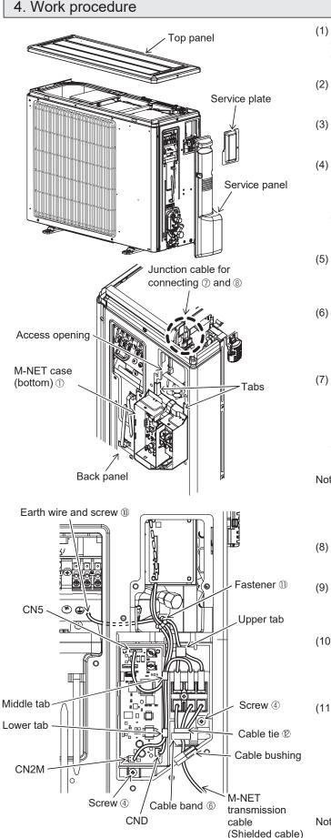
(1) Remove the top panel, service panel, and service plate.
