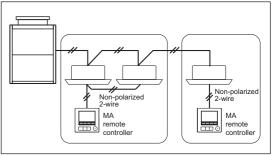
\*When this MA remote controller is connected to a group, no other MA remote controllers can be connected to the same group.
