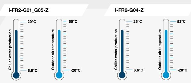
i-FR2-Z can operate with outdoor temperature down to -20°C and up to 52°C (50° for G01 and G05 units) and chilled water temperature from 6,6°C up to 25°C (20°C for G01 and G05 units).
