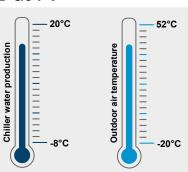
i-FX2-Y can operate with outdoor temperature down to -20°C and up to 52°C (50° for G01 and G05 units) and chilled water temperature from +20°C down to -12°C (-8°C for G04 units).
