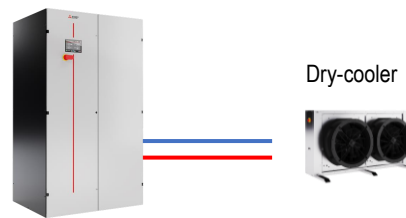
Direct Expansion, water cooled + FC coil – DW FC
