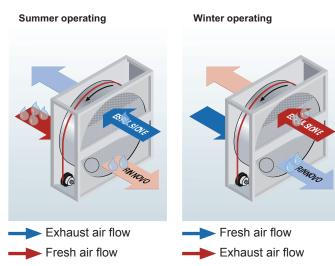
Additional filters are fitted to protect the heat exchanger from excessive fouling: in particular, class G4 filters are installed in the outside and exhaust air flow.
