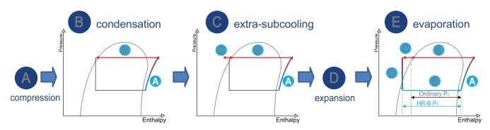
In winter mode evaporation phase is divided between external and booster coil. The favourable conditions of the exhaust air can be exploited to evaporate a certain amount of refrigerant with an higher temperature (C+) and therefore increase unit efficiency.
