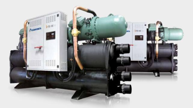
i-FX-W is the Climaveneta brand water cooled chiller with 1+i innovative logics that combines fifixed speed and variable speed screw compressors, thus ensuring continuous modulation of loads and a perfect leaving water stability.
