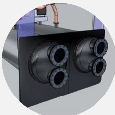
Heat exchangers with horizontal alignment
