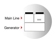
Redundancy increases uptime. FR2-G04-Z chillers also extend this concept to the electrical supply: the unit, equipped with an ATS\*, can be connected to two separate power lines to enhance the system's dependability.
